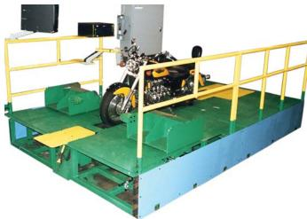
During the Low Speed Brake Test, the 10" rear roll clutch on both decks is
