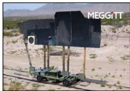
The MDS Caswell MAT vehicles are used to simulate a tank or other vehicle for live fire training and qualification programs. It provides training in detecting, identifying and firing upon moving tank targets under simulated combat conditions and is capable of lifting all full-scale flank targets.
